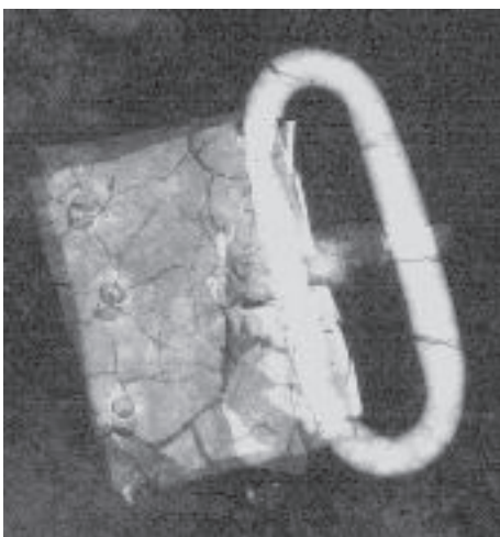
Fig 19 Bronze buckle from an early medieval grave. The buckle is fissured and very fragile and now comprises mostly tin oxide and copper carbonate. This is a consequence of decuprification of the bronze in the acid burial environment. Length: 21mm.
