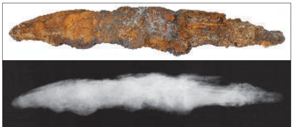
Fig 4 Early medieval knife with horn handle and leather sheath. The junction of the handle with the blade is clearly visible in the X-radiograph owing to iron mineralization of the different organic layers. Part of the handle is visible in the radiograph where the horn has been preserved by mineralisation on the tang. The sheath shows as an irregular and discontinuous line around the blade and also where it extends over part of the handle. Length: 170mm.
