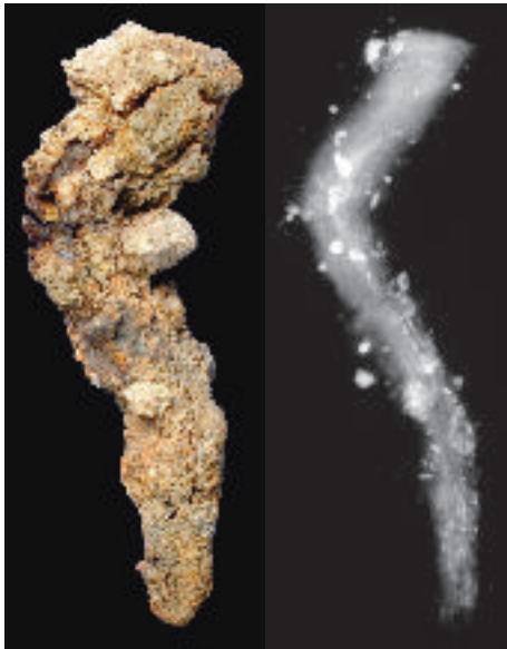
Fig 18 Medieval nail. The X-radiograph shows non-ferrous metal casting waste trapped within the corrosion layers. Length: 65mm.
