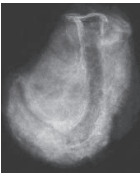
Fig 20 Roman nail, completely corroded. The X-radiograph reveals a void within the accreted block.
