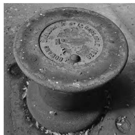
Fig. 71. BB96/03865. Devonport South Yard South Smithery (S126) photograph of Cowans Sheldon driven capstan (1926) (29 Feb 1996). ©Crown copyright.HE.
