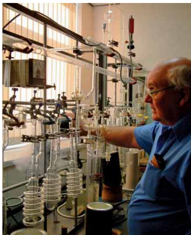
Fig 12 cleaning carbon dioxide prior to benzene synthesis
