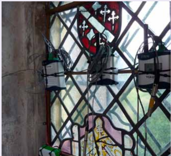
Monitoring the microclimate at Great Melford, Suffolk as part of the protective glazing research project (2A2). Photo Chris Wood, © English Heritage
