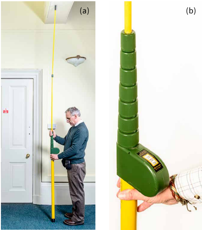
Figure 10 Telescopic measuring pole, extended to take a height measurement of the beam overhead (a) and a detail of the height measurement instrument (b).
