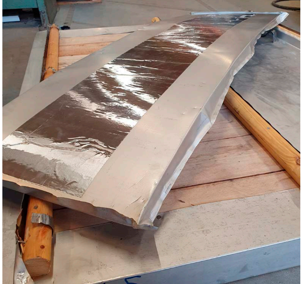
Figure 9: Acoustic mat bonded to underside of roofing for acoustic test
