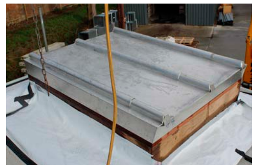
Figure 6: Round batten-roll roof sample under test
