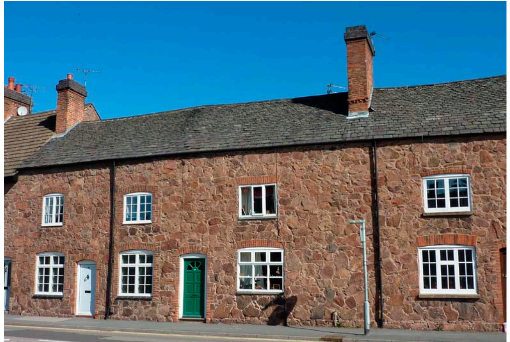
Figure 20: Cottages, Quorn. Mountsorrel Granodiorite with Swithland Slate roof.
