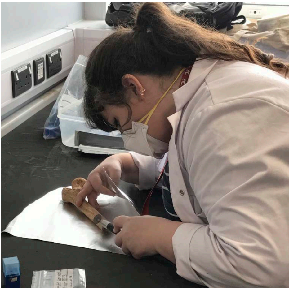
Fig 1 A sample being cut from a femur for radiocarbon dating. The small rotary electric saw is being used to remove the sample.
